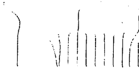
Fig. 4: Skeleton of the signal after denoising by g_2 wavelet. Comparing to Fig.2 (right) shows the disappearance of all short noise fractions smaller than a = 2 .
